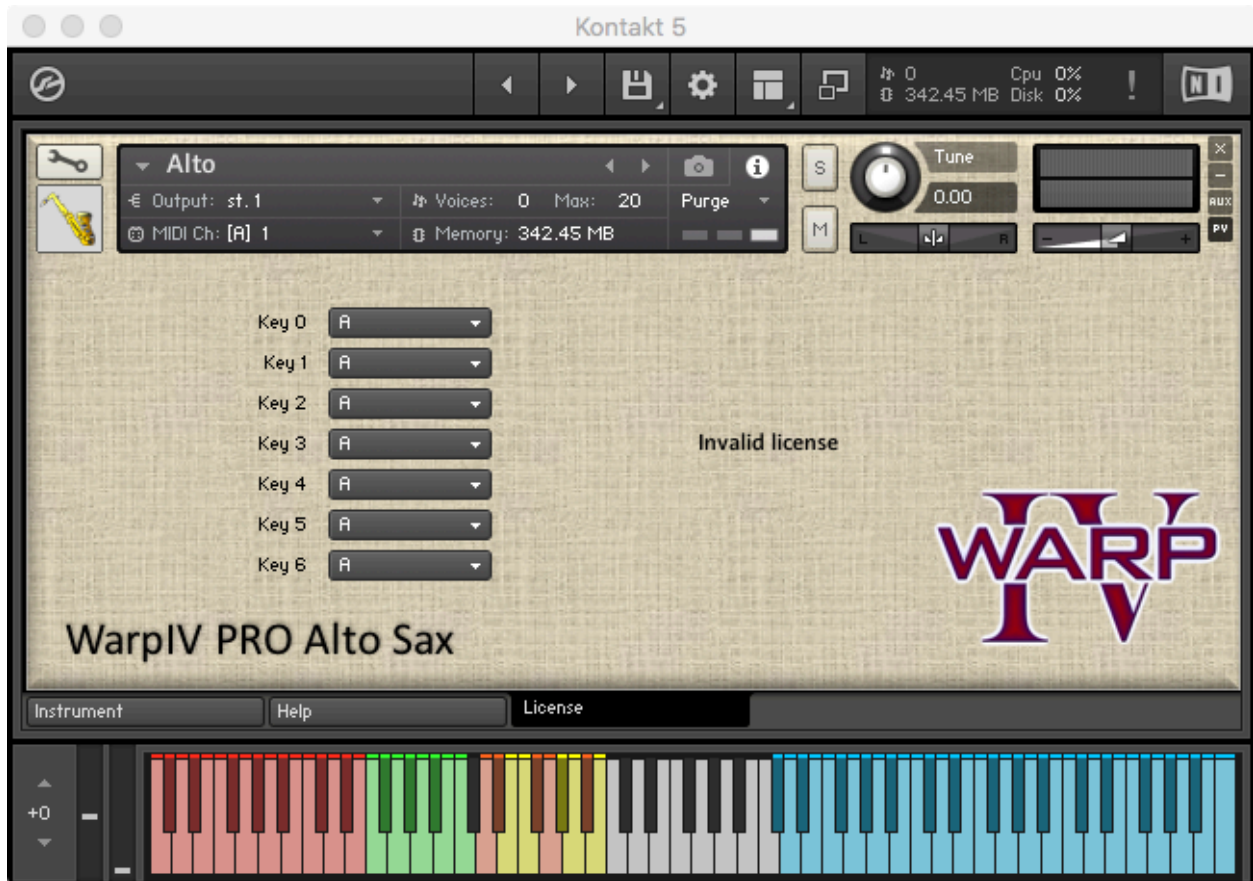
Figure 1: Setting your license key is accomplished by setting Key 0, Key 1, etc. to the values sent to you by email. Remember to resave your instrument so that you will not have to reenter it again.
